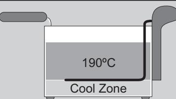
This type of fryer is only suitable for use with oil or liquid fat, and not with solid fat. Using solid fat entails the risk of trapping water in the fat which will cause it to spatter violently when heated up.
